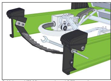
2. Using a 1/8" Allen wrench and 3/8" wrench, remove and discard the old pole strap and hardware. Move ahead to step 5.
