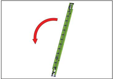
1. Lay the ladder down with the fly section facing the ground. If the pole strap is being added to the ladder skip to step 3.
