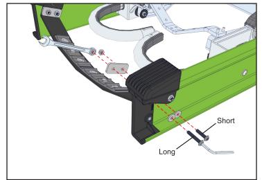
5. Align the new pole strap with the holes, then using a 1/8" Allen wrench and 3/8" wrench, tighten the new fasteners in the order shown. Make sure the long screw is closest to the end of the rail.
