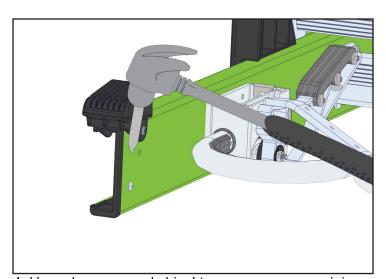
4. Use a hammer and chisel to remove any remaining rivet head material. Be careful not to damage the fiberglass rail.
